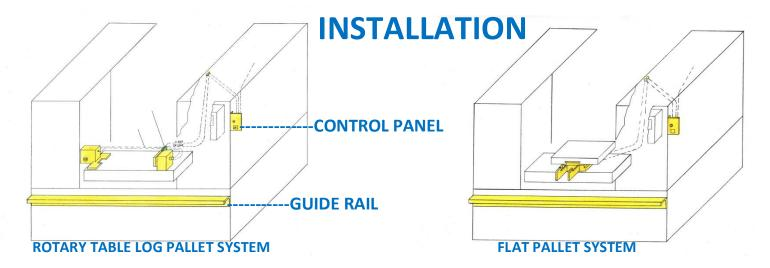
Installation of the Rotary Log Pallet System or the Flat Pallet System requires the mounting of a Guide Rail and a control panel. The guide rail locates the carts and enables them to position for pallet transfer.
