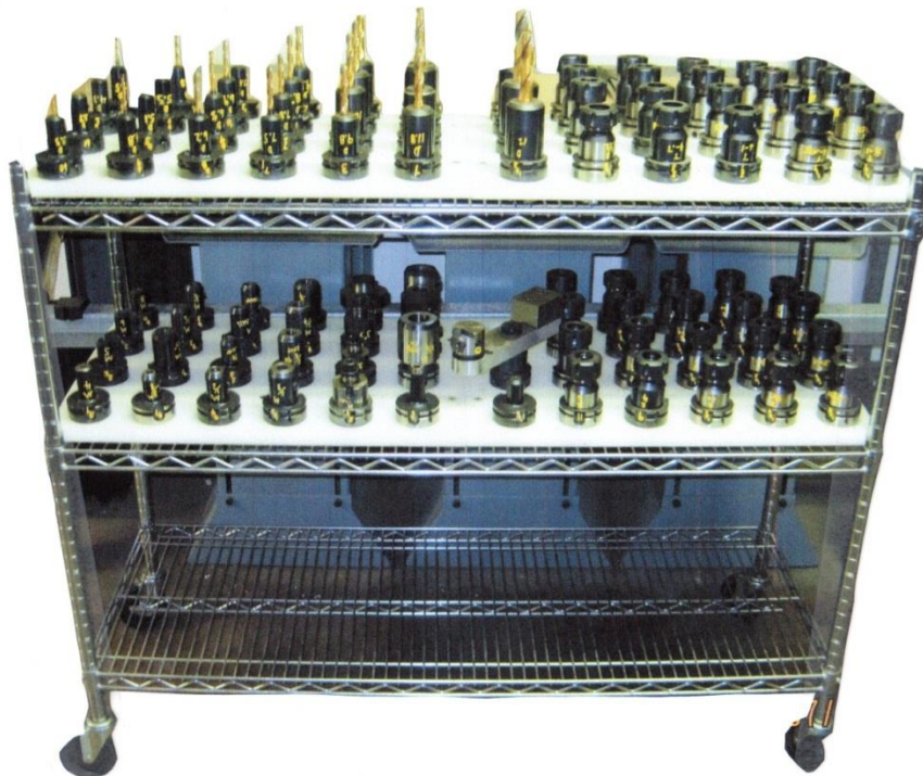
Example of a tool holder storage cart.
